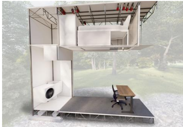
Figure 1-14: The NewVistas living module provides an individual with about 60 square feet of personal space, including a bedroom, bathroom, workstation, and other amenities. Two of these modules comprise a unit that can initially serve as an RV trailer or ADU and ultimately be connected into an apartment building.
